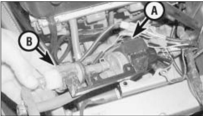
2.9c Fuel pump (A) and filter (B) are mounted in the fuel line from the tank to carburetors
