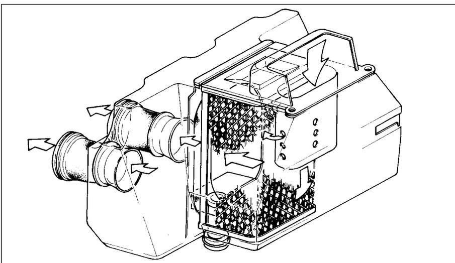
2.10c Section view of typical air filter housing
