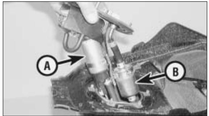
2.9d Fuel pump (A) and filter (B) mounted inside the tank
