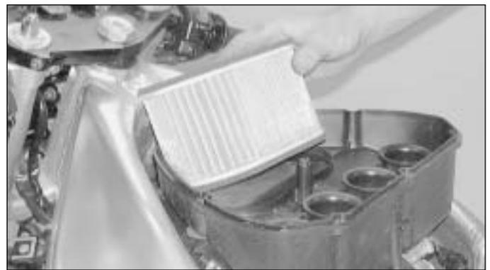
2.10b A pleated paper type filter as used on Yamaha's R1
