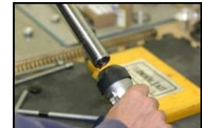
8. Push dampening rod in with your finger to remove it.
