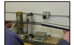
11. Begin putting the forks back together by standing them upright. Place the outer leg on top. Use the OEM bottom fork bolt with washer and tighten. (Recommended 15' lbs. of torque pressure)
