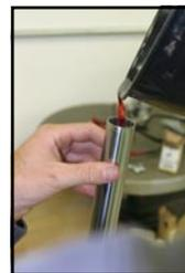
13. Firmly pump oil into fork and re-insert spring.
