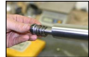
9. Use the OEM damping spring and OEM piston ring on the new TBR Piston.
