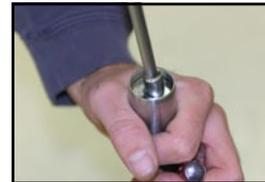
5. Keep fork leg upright (so that fork oil does not spill out) and remove the spring.
