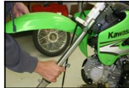
4. Remove the dust covers from the top of each leg and push down to remove the circlip. (Caution: The fork is spring loaded so carefully apply pressure from the top so that the spring does not pop out.)
