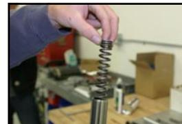
6. Firmly pump fork several times to remove fork oil. (If you are not re-using this oil, please dispose of it properly.)
